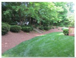
The rear yard slopes toward the home and there is evidence of erosion of soil along the sides yards that is directing drainage against the perimeter of the home. Corrections are needed to control drainage and prevent water penetration, a licensed general contractor should be consulted for a complete evaluation and to make necessary repairs.
